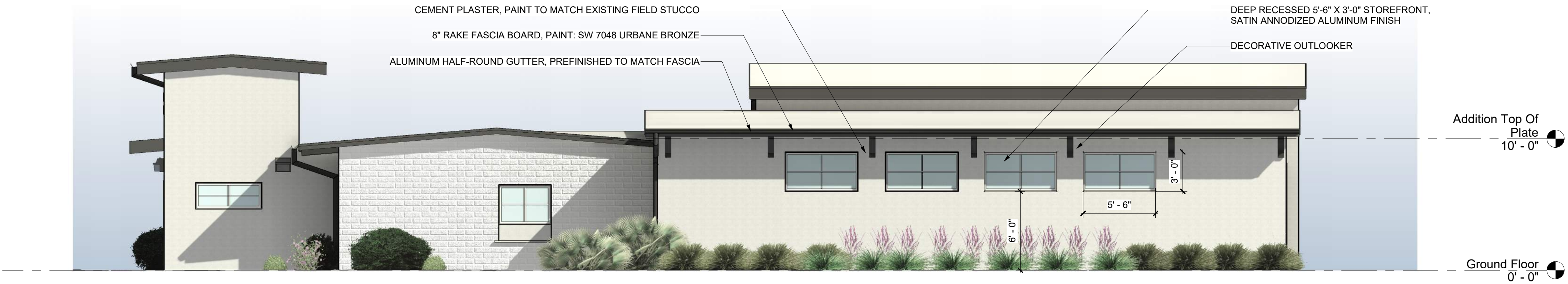
SOUTH ELEVATION - IMPROVEMENT 1 3/16" = 1'-0"
