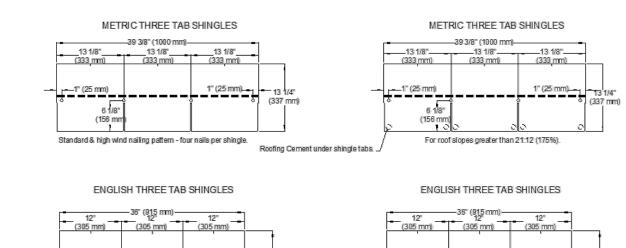
Roofing Cement under shingle. FIGURE 1—SHINGLE PROFILES AND FASTENER PATTERNS
