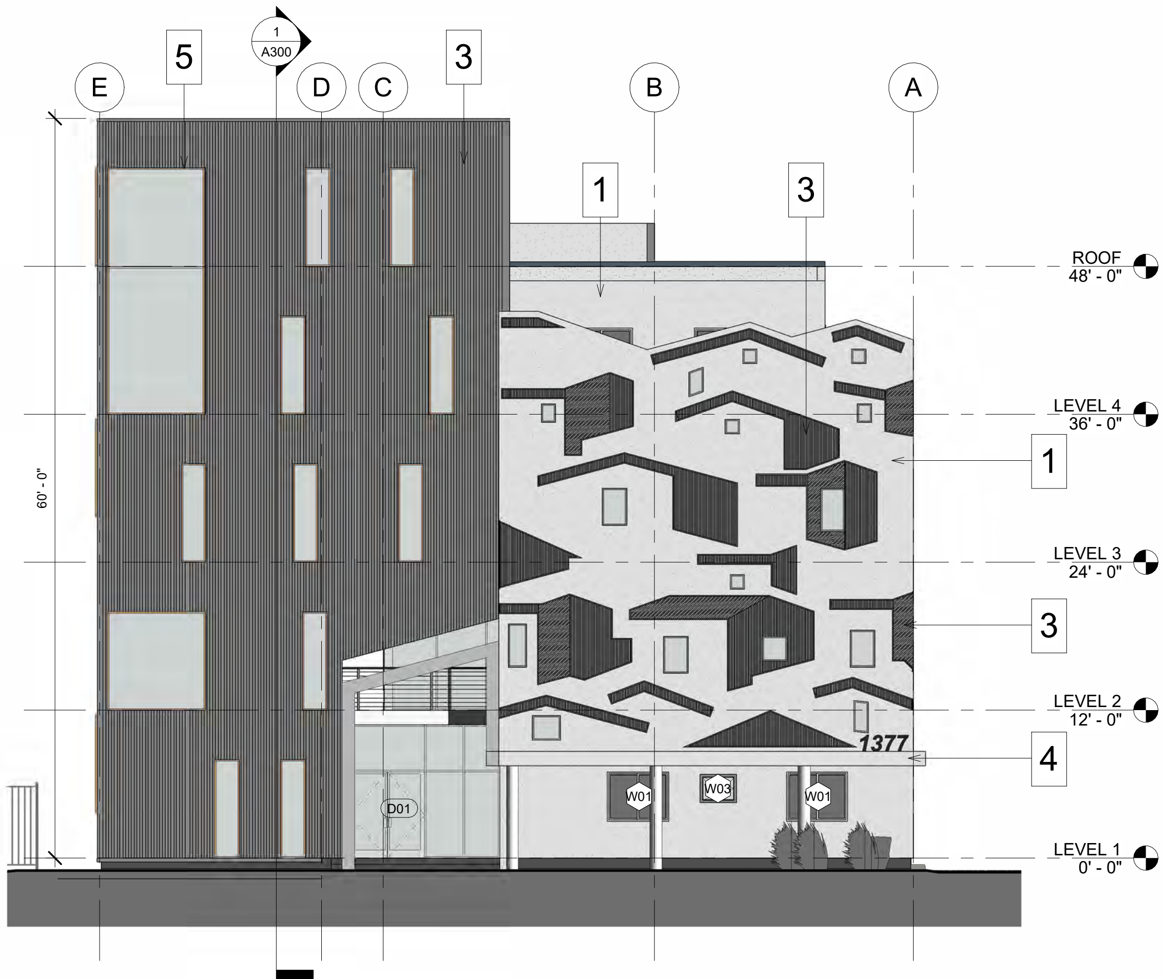
2 EXTERIOR ELEVATION - EAST 1/8" = 1'-0"
