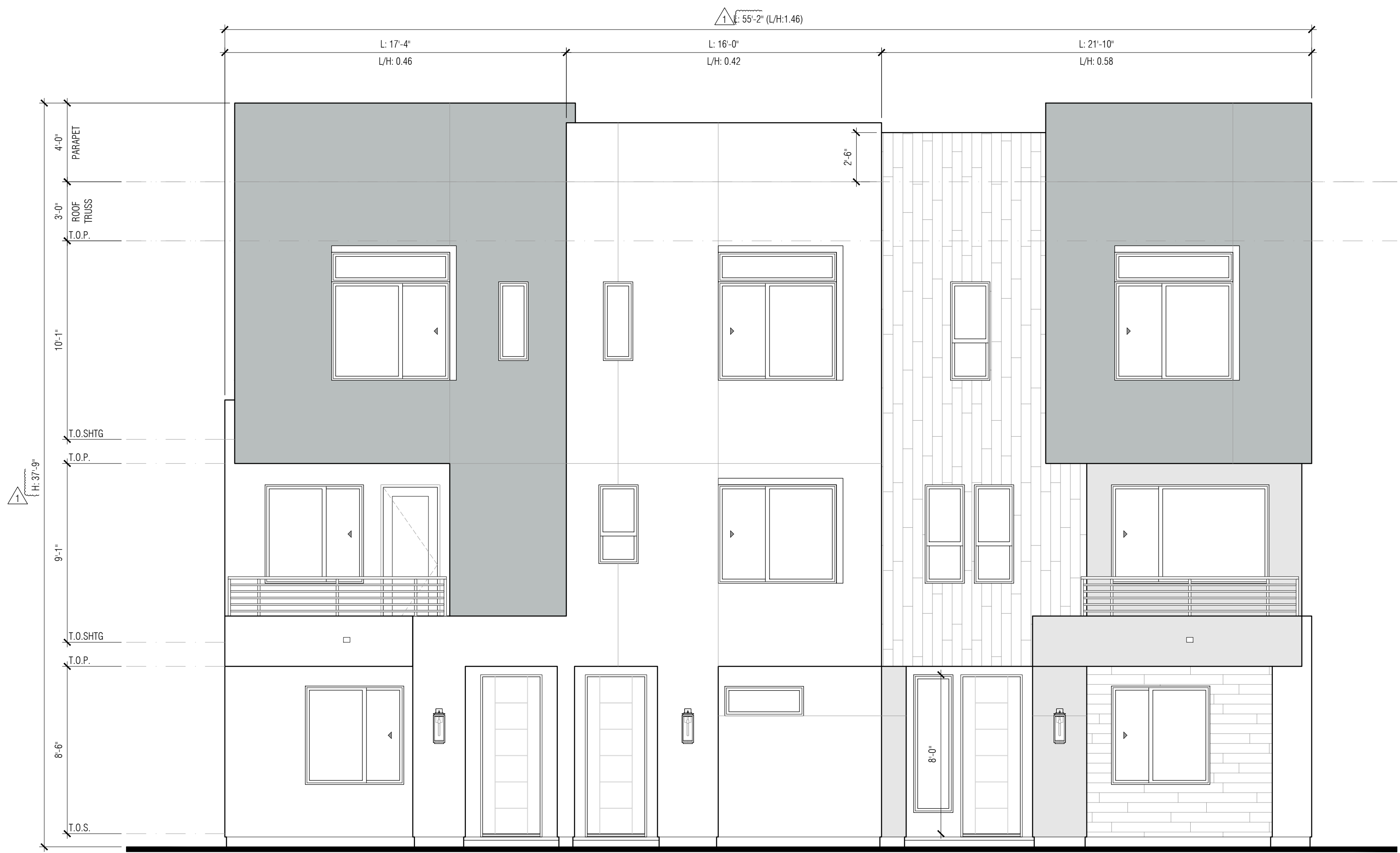
ENTRY SIDE BUILDING ELEVATION
