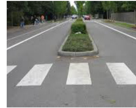
INSTALL RAISED MEDIAN ON APPROACHES
