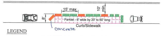
K-Rail (min. weight 1,500 lbs); Concrete or Water-fill
